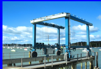
New 50 Tonne Travel Lift
